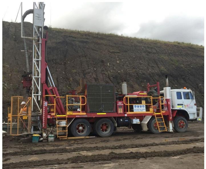
Drill to be used for groundwater monitoring on site
