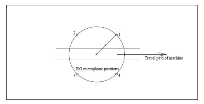
Figure 1 Sound power microphone positions
