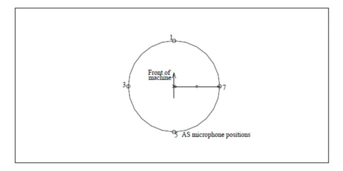
Figure 2 Alternative stationary sound power microphone positions
