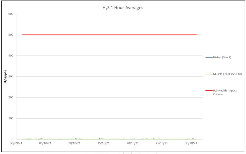
Figure 5: Hydrogen Sulphide 1 Hour Results
