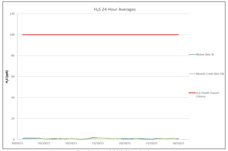
Figure 7: Hydrogen Sulphide 24 Hour Results
