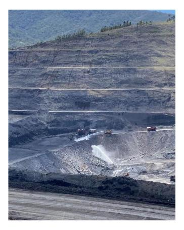
Photo 3 – Water carts located in Open Cut Mine 1 controlling minor spontaneous combustion
