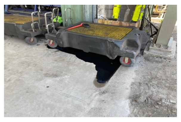
Photo 9 – Unattended hydrocarbon spill located in refuelling area
