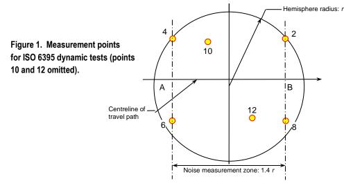
Measurement points 2 and 4 (6 and 8) were combined into a single point and the measurement zone extended to approximately 2.8 r to allow for an approach distance of 1.4 r to represent the measurement at point 2 (4) and a departure distance of 1.4 r to represent the measurement at point 6 (8).
